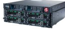
VIPRION 2400 2 x Quad core CPU x 4 Blade 4 Slots Chassis , 4U Size 320 Gbps L4/L7 Traffic
